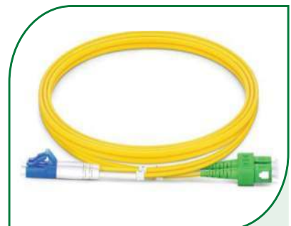
(1, 2, 3, 5, 10, 15, 20, 25, 30) M SINGLE MODE SC/APC - LC/UPC DUPLEX FIBER OPTIC PATCH CORD LSZH
